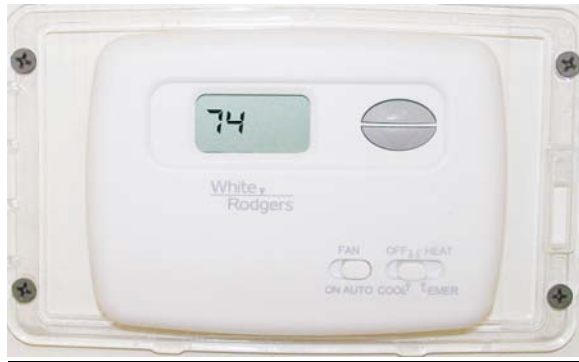
Off, Switch Set to Position 1
